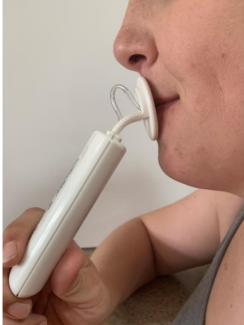
Figure 11 Tongueometer™ use with lip guard. Bulb tubing passes through lip guard and is held firmly in place
